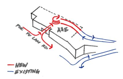
The future AED shall be on the whole floor at a podium level, with the pathology floors below facing the sea. Other "hot floors" could be positioned immediately above the AED and then the programme floors on top (see **Figure 10**).
