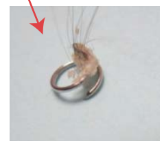
Broken tip of fetal scalp electrode
