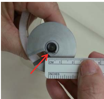
Small fragment found missing
